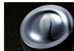
Metal mold for producing the aspherical lens
